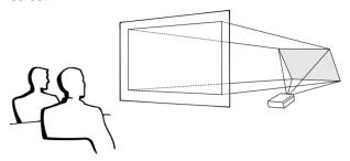
NOTE Optimal image quality is produced with the unit positioned perpendicular to the screen with all feet flat and level.
