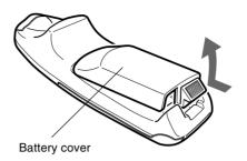
2 Insert the two supplied batteries (size AAA/R03). Ensure that the polarities (+ and -) of the batteries are aligned correctly.
