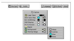
This function allows you to select the image displayed when no signal is being sent to the projector.
