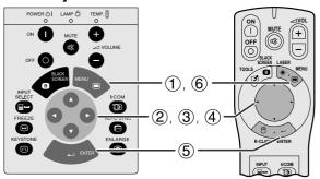
When displaying computer patterns which are very detailed (tiling, vertical stripes, etc.), interference may occur between the LCD pixels, causing flickering, vertical stripes, or contrast irregularities in portions of the screen. Should this occur, adjust "Clock", "Phase", "H-Pos" and "V-Pos" for optimum computer image.
