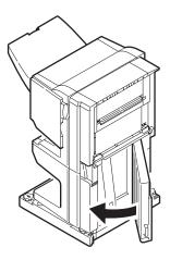
**10.** Move the Finisher and Inverter back into position and connect to the printer.
