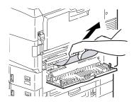
**4.** Put the paper guide back into position and close Tray 1 side cover.
