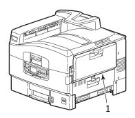
2. Pull the release lever (2) and pull open the side cover.
