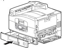
Sharp AR-C360P User's Guide Consumables and maintenance > 50 **6.** Return the paper guide plate to its original position and close Tray 1 side cover.
