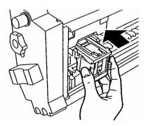
**11.** Ensure that the staple cartridge is securely installed back into the staple unit then push the staple unit fully home.
