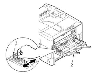
**3.** Adjust the paper guides (3) to the size of the paper being used.
