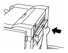
**5.** Check that the punch chip box has been replaced correctly then move the Finisher back into position, being careful not to trap your fingers.
