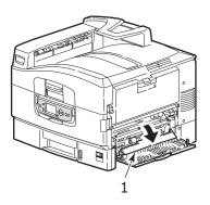
Sharp AR-C360P User's Guide Consumables and maintenance > 49 **3.** Remove Tray 1 completely from the printer.
