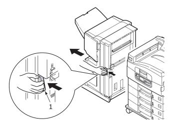
Sharp AR-C360P User's Guide Troubleshooting > 68 **2.** Operate the duplex cover release button (2) and open the cover.
