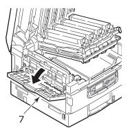
**8.** Open the side cover (paper exit) (8) and remove the jammed paper.
