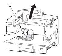
To close the top cover, push gently (1) until the cover stops midway and then push harder (2) to close the cover completely. Ensure that the cover is securely closed.
