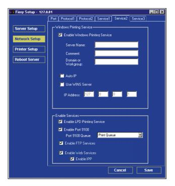
**Enable Windows Printing Service**—Select to enable SMB (Server Message Block), the file and printer sharing protocol built into Windows. Enabling SMB lists the Fiery on the network so that Windows clients can print to a particular print connection (Hold, Print, or Direct) on the Fiery without any other networking software. For information on setting up a Windows client for Windows printing, see the *User Software Installation Guide*.
