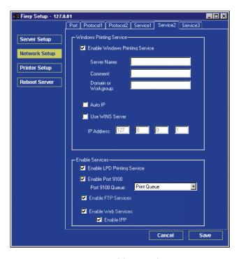
Enable Port 9100—Enables applications to open a TCP/IP socket to the Fiery at Port 9100 to download a print job.
