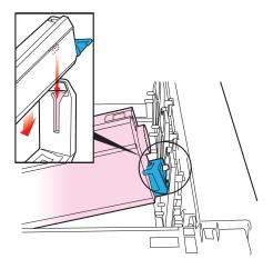
**6.** *Gently* push the colored lever toward the rear of the machine until it stops. This releases the toner into the image drum.
