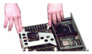
**b.** Align the module with the narrow strip (1) on its metallic contact edge to the right (toward the slot identifier numbers ) of the control board.
