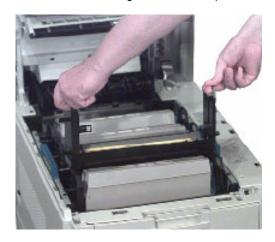
**6.** Push the tab inwards and remove the blanking plate from the image drum.
