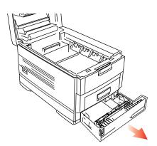
**3. Check behind the front cover.** Open the front cover and remove any jammed paper, then close the front cover.
