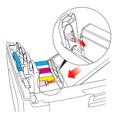
**7.** *Gently* push the toner cartridge down, engaging the locking pin into the groove on the image drum.
