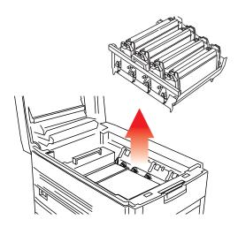
**3.** Press back the lock lever (1) and, using the handles (2 and 3), remove the old transfer belt from the printer.
