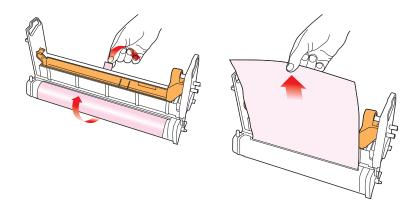
**5.** Install the new image drum in the printer.
