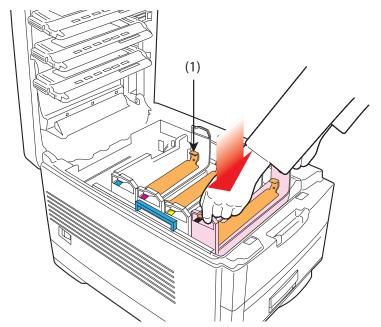
**7.** Push the tab (1) inwards and remove the blanking plate from each of the image drums.
