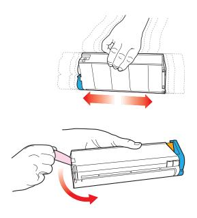
**3.** Remove the locking piece from behind the colored toner release lever.
