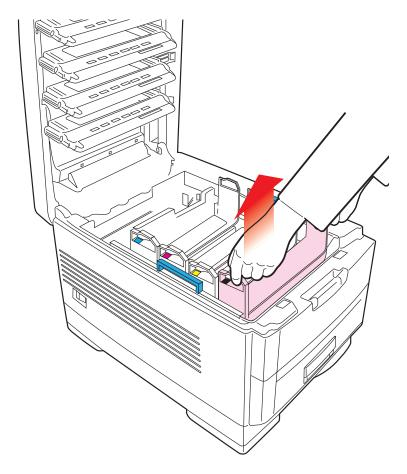
**4.** Seal the aperture on each image drum and its toner cartridge with plastic adhesive tape (1) to prevent any toner spillage during transportation.
