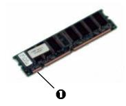
c. Carefully insert the module in the socket, placing the ends into the slot in the lock tabs. Press down firmly, until you feel the board engage the connector, then make sure the white tabs come up to lock the module in place.
