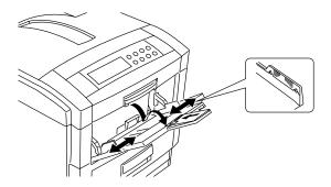
**2.** Load the media face *up*, and adjust the paper guides to the size of the media being used.
