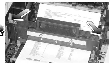
c. Re-lock the levers at either end of the fuser.
