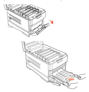
**b.** Open the duplex top cover and remove any jammed paper.
