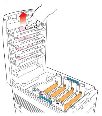
**4.** Remove the four image drums and place them on a level surface.
