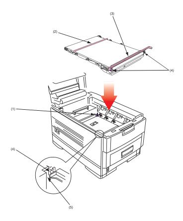
**6.** Move the lock lever (1) toward the front of the printer and ensure it locks the transfer belt into place.
