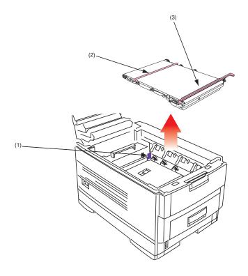
**4.** Remove the new transfer belt unit from its packaging.
