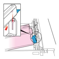
**8.** *Gently* push the colored lever toward the back of the printer until it stops. This releases the toner into the image drum.
