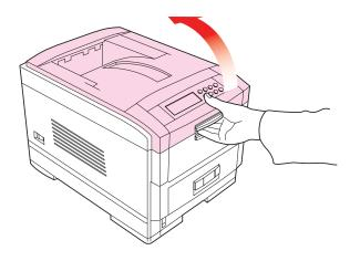
2. Remove the cradle complete with the four image drums and toner cartridges from the printer.
