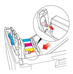
**5.** *Gently* push the toner cartridge down engaging the locking pin into the groove on the image drum.
