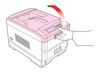
**2.** Remove the appropriate image drum/toner cartridge from the printer.
