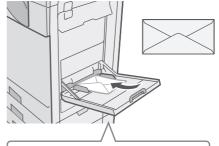
Only the address side of envelopes can be printed on. Place envelopes with the address side face down.
