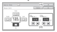
(3) Select 3/4" for the front side and 3/4" for the reverse side using the
