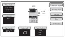
To use a special mode, open the special modes menu and touch the key of mode that you wish to use. The menu consists of two screens. Use the keys to switch between the screens.
