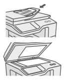
If the X dimension (width) of the document is less than 3-1/2" (89 mm) or the Y dimension (height) is less than 4" (100 mm), place the original on the document glass.
