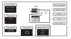
To select paper, touch the [Paper Select] key or the image of the machine in the base screen of copy mode.
