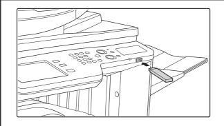
Connect the USB memory device to the machine.
