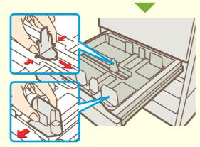
Move the two guides on the tray to change the size from 8-1/2" x 14" (B4) to 8-1/2" x 11' (A4).
