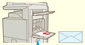
Only the address side of envelopes can be printed on. Place envelopes with the address side face down.
