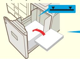
Load paper in the large capacity tray as shown. The size of paper used in the large capacity tray can only be changed by a service technician.
