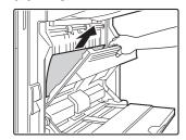
Open the Paper reversing section cover and remove the misfed paper.
