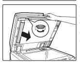
Open the automatic document feeder. Rotate the transfer roller in the direction of the arrow and remove the original.
