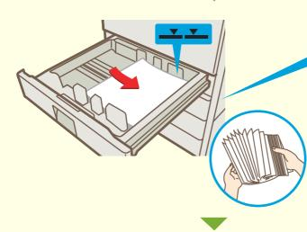
Insert the paper with the print side face up. Fan the paper well before inserting it. Otherwise, multiple sheets may feed at once and cause a misfeed.
