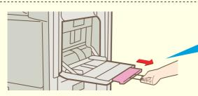
When loading 12" x 18", 11" x 17", 8-1/2" x 14", or 8-1/2" x 13"R size paper, pull out the tray extension. The maximum number of sheets that can be loaded in the bypass tray is approximately 100 for plain paper and approximately 20 for postcards.
