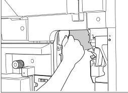
Pull the lock lever to the front until the automatic duplexer comes to a stop.
