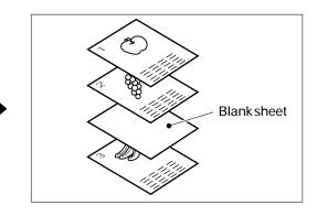
• Inserting a copied special sheet at the specified page number
