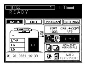
$\label{eq:press} \begin{array}{l} \mbox{Press the } \underline{2 \rightarrow 1} \mbox{ key to select the function} \\ \mbox{of single-sided copies from two-sided} \\ \mbox{originals.} \end{array}$
