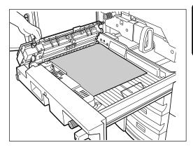
Push the lock lever and open the transport unit cover.
