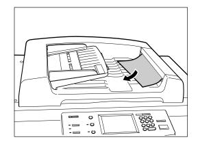
Open the ADF exit cover and remove any foreign matter such as bits of paper, paper clips, etc.
