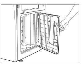
Note: If you want to add paper before the largecapacity feeder runs out of paper, press the TRAY DOWN 🕞 key before opening the door. The elevator tray will automatically move down.
