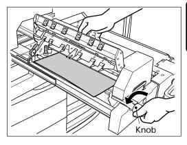
**13** Return the transport-belt unit until it comes to a stop and turn the knob clockwise to lock the lever.
