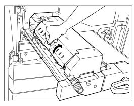
• If any paper is found, turn the knob counterclockwise and remove it as shown.
