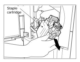
Pull out the staple guide with the knob (2) while pushing the blue lever (1).
