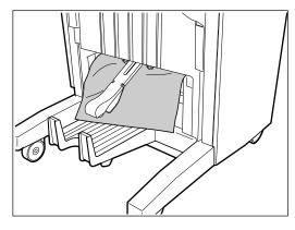
If necessary, open the exit cover of the saddle stitcher and remove any misfed paper.
