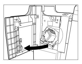
2 Turn the blue lever 90 degrees to the left and pull out the stapler unit.
