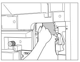
Turn the knob counterclockwise and pull out the transport belt until it stops.
