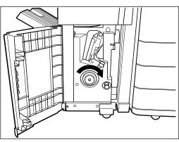
Remove the paper misfed on the exit side of the saddle stitcher.
