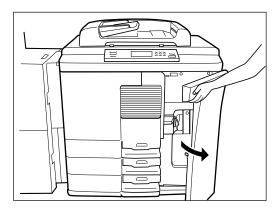
2 Grip the lock lever to unlatch it and move the large-capacity feeder to the right slowly until it comes to a stop.
