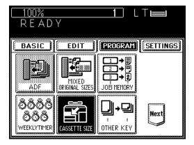
2 Select the cassette to be reset, then press the COVER or INSERT key on the bottom right and check that the cassette is reset to the previous paper size.
