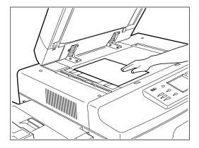
When the first original has finished being scanned, press the YES key, set the next original and press the START key.
