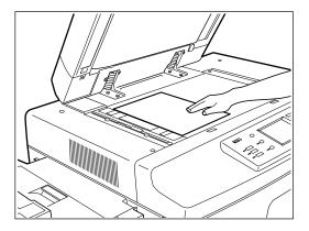
When the first original has finished being copied, place the next original and press the START key.
