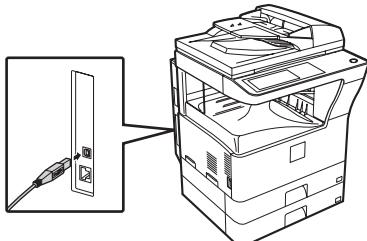
**2** Insert the other end of the cable into your computer's USB connector.
