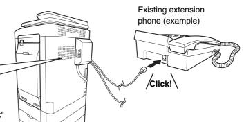
• Connect an extension phone that has a modular jack. Use standard phone line cable to connect the phone. If other than a standard phone line cable is used, the connection may not work correctly.
