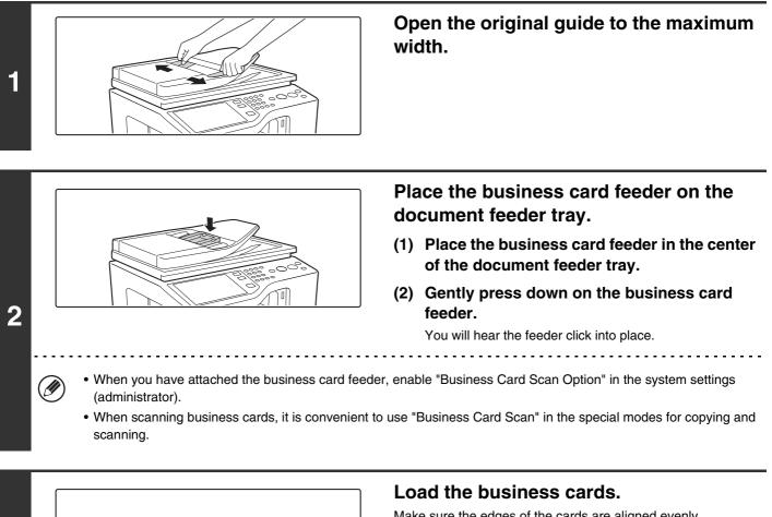
Make sure the edges of the cards are aligned evenly. Insert the cards face up all the way into the business card feeder.
