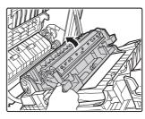
If the misfeed is not in the above location, grasp the handle on the secondary transfer roller unit, slowly open the unit, and remove the paper.
