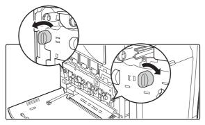
(2) Grasp the lock levers and tip the cover forward.
