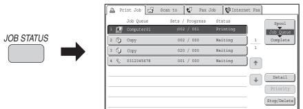
The job status display (A) is in the lower left corner of the touch panel. The job status display can be touched to display the job status screen. You can check the first four print jobs in the print queue (the job in progress and reserved jobs) in the job status display (B).
