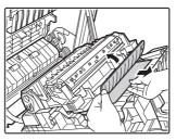
Open the right side cover, open the paper conveyor cover, and remove the paper.
