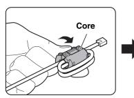
Attach the provided core to your extension telephone cord and then connect the cord to the machine.
