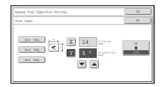
Touch the [X] key and enter the horizontal dimension of the paper with the  $\frown$  keys, and then touch the [Y] key and enter the vertical dimension. When finished, touch the [OK] key.
