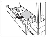
When a paper gets twisted to the roller, remove the tray and remove the misfeed paper.
