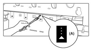
(2) Insert the cleaning tool all the way into the hole and then pull it back out.
