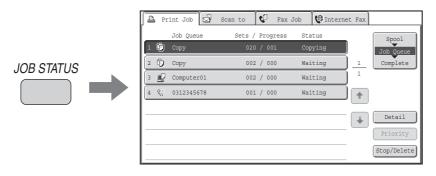
The job status display (A) is in the lower left corner of the touch panel. The job status display can be touched to display the job status screen. The first four jobs in the print queue (the job in progress and reserved jobs) can be checked in the job status display (B).
