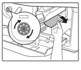
Turn roller rotating knob in the direction of the arrow to remove the misfed paper.
