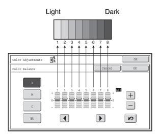
Each of the colors yellow, cyan, magenta, and black are divided into 8 gradations from light to dark, and the average density of each gradation can be adjusted, or all eight gradations can be adjusted at once.
