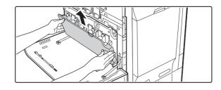
Remove the cleaning tool for the writing unit from the front cover.
