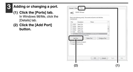
To change to a previously created port such as USB port, select the desired port (USB001, etc.) from the list and click the [Apply] button. This changes the port.
