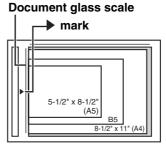
All originals should be placed in the left center position. Align the middle of the original with the tip of the **b** mark.
