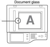
When using the staple sort function, place the original so that the top of the image is toward you.
