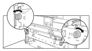
(2) Grasp the lock levers and tip the cover forward.
