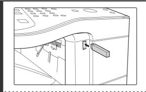
Connect the USB memory device to the machine.
