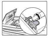
Lift up the knob that holds the roller shaft.
