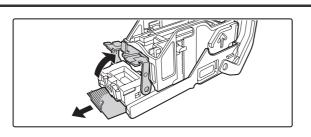
Raise the lever at the front end of the staple case and remove the jammed staple.
