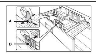
Adjust the guide plates A and B by squeezing their lock levers and sliding them to match the vertical and horizontal dimensions of the paper to be loaded.
