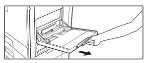
When loading paper larger than 8-1/2" x 11" or A4, be sure to pull out the bypass tray extension. Pull the bypass tray extension all the way out. If the bypass tray extension is not pulled all the way out, the size of the loaded paper will not be correctly displayed.
