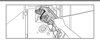
Pull the staple unit of the saddle stitch finisher forward and then rotate it back to its original position. 7
