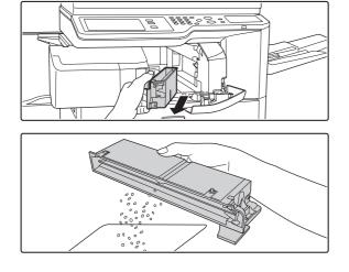
Grasp the punch waste box handle, gently pull out the box, and discard the punch waste.
