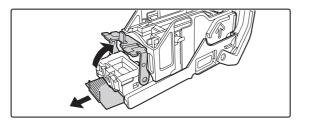
Raise the lever at the front end of the staple case and remove the jammed staple.
