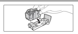
Insert a new staple cartridge into the staple case as shown.
