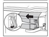
While pressing the lever over to the left, slide the finisher to the left until it stops.
