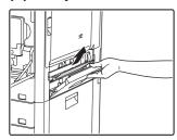
The misfeed may have occurred inside the machine. Check carefully and remove
