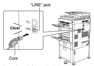
Insert the end of the cord with the core into the "LINE" jack.
