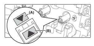
Insert so that the cleaning location label (A) and the charger cleaner label (B) are oriented as shown.
