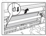
Lower the lever in the direction of the arrow to remove the misfed paper.
