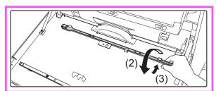
(2) Place the right-hand side of the cleaning instrument on the front side, spread across the top of the claw.
