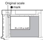
Set an original by aligning its corner with the tip of the scale (★) mark at the left rear corner of the glass as shown in the illustrations.
