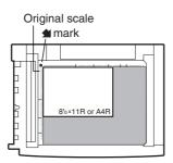
Set an original by aligning its corner with the tip of the scale (1) mark at the left rear corner of the glass as shown in the illustrations.
