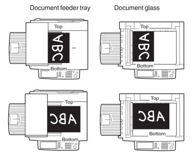
Place originals in the document feeder tray or on the document glass so that the top of the original is positioned to the rear side of the machine. If not, staples will be incorrectly positioned and some special features may not give the expected result.
