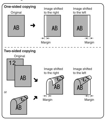
The shift direction can be selected from right or left shift as shown in the illustration.
