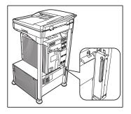
The part indicated in the illustration is only to be handled by a service technician. Absolutely do not touch this part.
