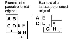
When making automatic two-sided copies of a one-sided 11" x 17" (A3) or 8-1/2" x 14" (B4) size portrait original, or when you wish to invert the top and bottom of the back side of a two-sided original, touch the [BINDING CHANGE] key.
