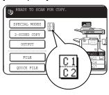
A corresponding icon representing the feature will appear on the touch panel and on the main screen of the mode selected. If this icon is touched, the setting screen of the function (or a menu screen) will
