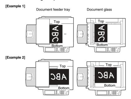
Place originals in the document feeder tray or on the document glass so that the top and bottom of the original is positioned as shown in the illustration. If not, staples will be incorrectly positioned and some special features may not give the expected result.
