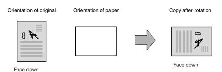
●This function operates in both the auto paper select or auto image mode. ("Rotation copy setting" can be disabled with a key operator program. See page 14 of the key operator's guide.)
