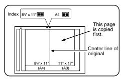
Place the opened original on the document glass so that the first page you wish to copy is on the right and the center of the original is aligned with the size mark.
