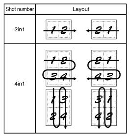
The arrows in the above diagram indicate the directions in which the images are arranged.
