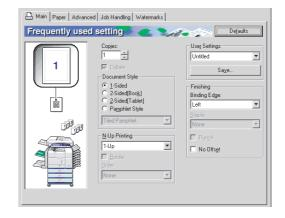
(1) To use a two-sided printing function, open the "Main" tab and select the desired two-sided printing radio button.
