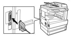
Insert the other end of the cable into your computer's parallel port.
