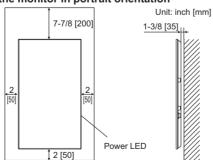
If it is difficult to provide sufficient space for any reason such as the installation of the monitor inside a housing, or if the ambient temperature may be outside of the range of 32°F (0°C) to 104°F (40°C), install a fan or take other measures to keep the ambient temperature within the required range.
