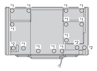
The cables connected to the terminals on the rear of the monitor and the USB cable on the back of the tray can be fastened with the cable clamp.
