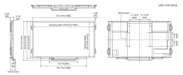
When mounting the monitor, be sure to use a wall-mount bracket that complies with the VESA-compatible mounting method. SHARP recommends using M6 screws and tighten the screws.
