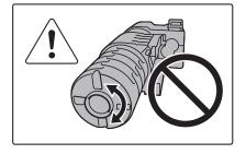
Shake the toner cartridge horizontally. Do not rotate it as shown at left.
