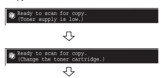
If you continue to use the machine without replacing the cartridge, the following message will appear when the toner runs out.
