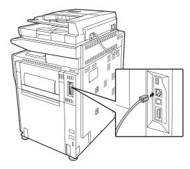
After connecting the machine to a network, be sure to configure the IP address and other network settings before installing the software. (The factory default setting for the IP address is to receive the IP address automatically when the machine is used in a DHCP environment.)
