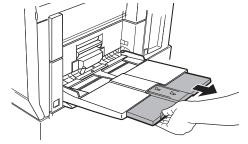
When loading 11" x 17", 8-1/2" x 14", 8-1/2" x 13", 8-1/2" x 11"R, A3, B4, or A4R size paper, pull out the tray extension.
