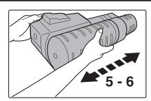
Remove the new toner cartridge from the box and shake it five or six times horizontally.
