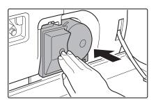
Push the cartridge in until it locks securely in place.
