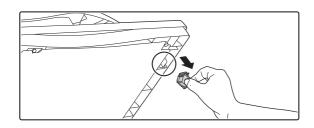
Open the automatic document feeder and remove the glass cleaner.
