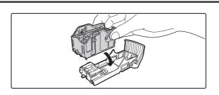
Insert a new staple cartridge into the staple case as shown.
