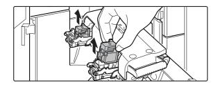
Grasp the left and right side of each empty staple cartridge and remove the cartridges.
