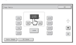
Touch a numeric value display key to directly enter a value with the numeric keys.
