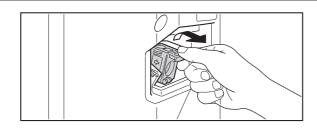
Squeeze the green parts of the staple case and pull the case up and then out.
