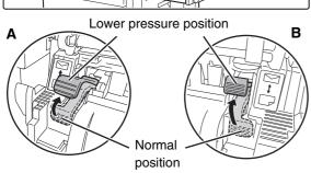
Move the fusing unit pressure adjusting levers (two) to the lower pressure position as shown.
