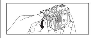
Lower the lever at the front end of the staple case and remove the jammed staple.
