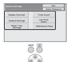
Use the arrow keys to select the desired item, press the [OK] key, and configure the settings.
