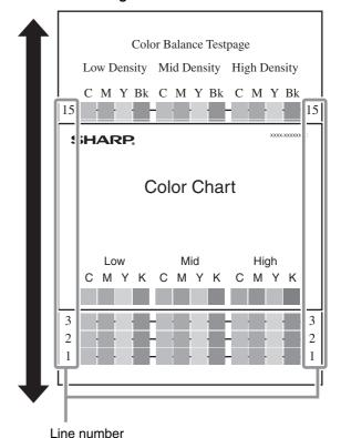
(5) Enter the line numbers recorded in step 4 in the C, M, Y, and Bk boxes of "Low Density", "Mid Density", and "High Density" in the Color Balance and click the [Submit] button.
