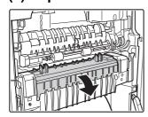
If a paper misfeed has occurred inside the fusing unit, press down on the green part, open the fusing unit, and remove the paper.
