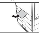
When a paper gets twisted to the roller, remove the tray and remove the misfed paper.
