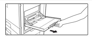
When loading paper larger than 8-1/2" x 11" or A4, be sure to pull the bypass tray extension all the way out. If the bypass tray extension is not pulled all the way out, the size of the loaded paper will not be correctly displayed.
