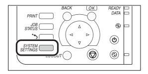
Make sure that the machine is in the standby state and then press the [SYSTEM SETTINGS] key on the operation panel.
