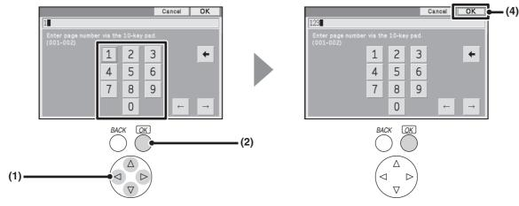
(1) Use the arrow keys to move the frame to the desired number.
