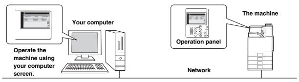
The remote operation function can only be used on one computer at a time.
