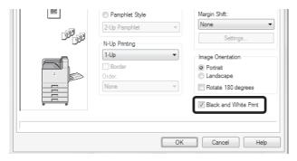
The [Black and White Print] checkbox on the [Main] tab and the "Color Mode" setting on the [Color] tab are linked. When the [Black and White Print] checkbox is selected on the [Main] tab, [Black and White] is also selected on the [Color] tab.
