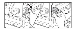
Lower the staple case release lever and remove the staple case.
