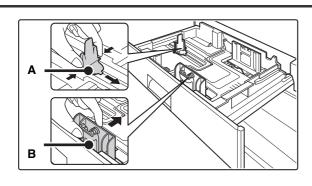
Adjust the guide plates A and B by squeezing their lock levers and sliding them to match the vertical and horizontal dimensions of the paper to be loaded.
