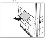
When a paper gets twisted to the roller, remove the tray and remove the misfed paper.
