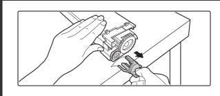
Remove the protective material from the new toner cartridge.
