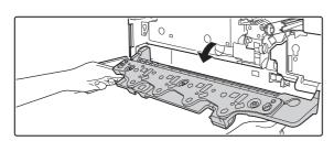
(2) Grasp the lock levers and tip the cover forward.
