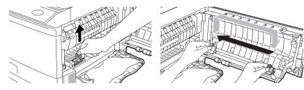
**4** Return the charger cleaner to its original position. Close the side cover by pressing the round projections near the side cover open button.
