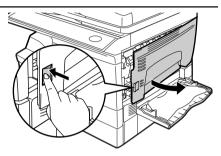
**3** Check the misfeed location. Remove the misfed paper following the instructions for each location in the illustration below. If the error indicator blinks, proceed to "A: Misfeed in the paper feed area" (p.102).
