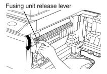
2 Gently remove the misfed paper from under the fusing unit as shown in the illustration. If the paper cannot be removed, proceed to "C: Misfeed in the transport area".
