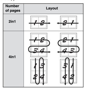
The arrows in the above diagram indicate how the images are arranged.
