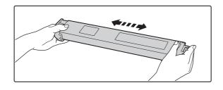
Remove a new toner cartridge from its package and shake it horizontally five or six times.
