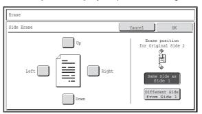
Touch the checkbox of the edge that you wish to erase and make sure that a checkmark ( ) appears.
