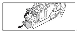
Raise the lever at the front end of the staple case and remove the jammed staple.
