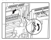
Rotate knob and remove the misfed paper.
