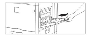
When loading a large sheet of paper, be sure to pull out the bypass tray extension. Pull the bypass tray extension all the way out.
