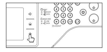
Make sure that the machine is in the standby state and then touch the [SYSTEM SETTINGS] key (�) on the touch panel.
