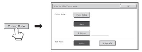
The following settings can be selected for the scanning color when the [COLOR START] key or the [BLACK & WHITE START] key is pressed.
