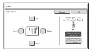
Touch the checkbox of the edge that you wish to erase and make sure that a checkmark () appears. When performing two-sided scanning, set the erase edge
