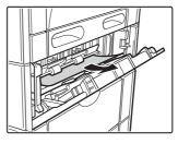
The misfeed may have occurred inside the machine. Check carefully and remove it.
