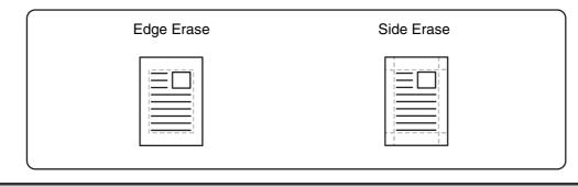
• Shadows at the edges of the original can also be erased when the automatic document feeder is used.
