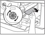
Turn roller rotating knob in the direction of the arrow to remove the misfed paper.
