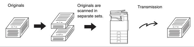
Up to 999 pages can be scanned. Note that when the memory is being used for other jobs, fewer pages can be scanned.
