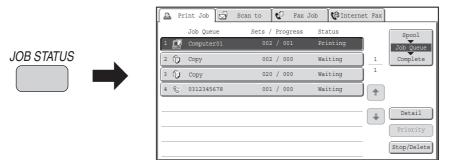
The job status display (A) is in the lower left corner of the touch panel. The job status display can be touched to display the job status screen. You can check the first four print jobs in the print queue (the job in progress and reserved jobs) in the job status display (B).
