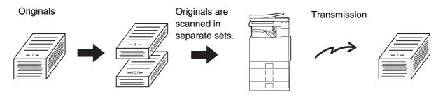
Up to 999 pages can be scanned. Note that when the memory is being used for other jobs, fewer pages can be scanned.
