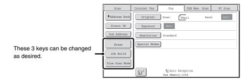
Displaying a program key in the base screen will enable you to call up the program by simply touching the key. STORING FAX OPERATIONS (Program) (page 4-66)
