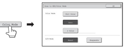
The following settings can be selected for the scanning color when the [COLOR START] key or the [BLACK & WHITE START] key is pressed.
