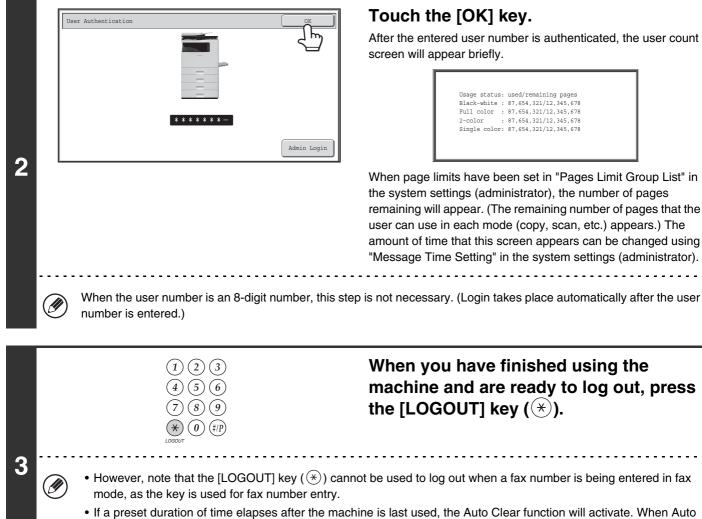
If a preset duration of time elapses after the machine is last used, the Auto Clear function will activate. When Auto Clear activates, logout takes place automatically. However, when PC Scan mode is used, logout does not take place when the [LOGOUT] key (\*) is pressed and Auto Clear does not operate. Change to a different mode on the machine and then log out.
