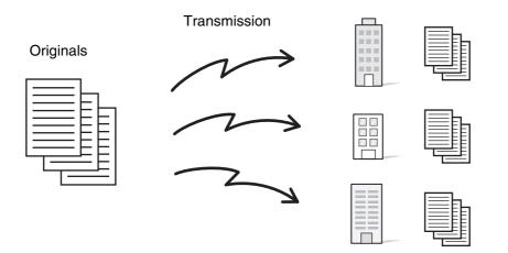
It is convenient to store destinations to which you frequently send faxes by broadcast transmission in group keys. Group dialing allows you to retrieve multiple fax numbers stored in a one-touch key by simply pressing the one-touch key. To store group keys, see "Address Control" (page 7-16) in "7. SYSTEM SETTINGS".
