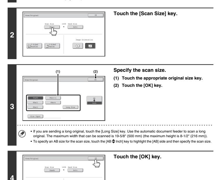
When [Long Size] is selected, the 2-sided scanning setting and send size cannot be changed. In addition, when only scan destinations are selected for scan transmission or metadata transmission, scanning will take place in Mono2.
