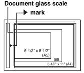
All originals should be placed in the left center position. Align the middle of the original with the tip of the hark.
