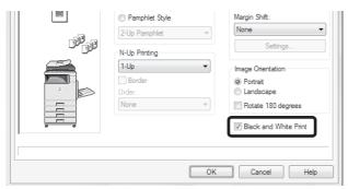
The [Black and White Print] checkbox on the [Main] tab and the "Color Mode" setting on the [Color] tab are linked. When the [Black and White Print] checkbox is selected  $\boxed{}$  on the [Main] tab, [Black and White] is also selected on the [Color] tab.
