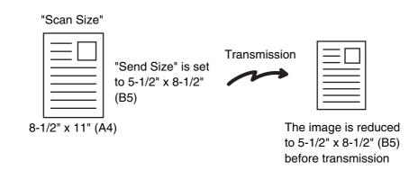
If the size of the placed original is different from the displayed original size, specify the original size.
