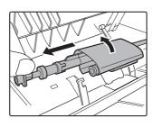
Remove the shaft rotating the roller cover upward and remove the shaft.
