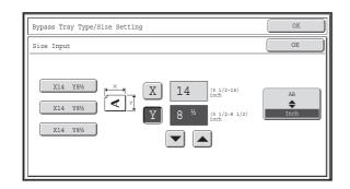
Touch the [X] key and enter the horizontal dimension of the paper with the  $\frown$  keys, and then touch the [Y] key and enter the vertical dimension. When finished, touch the [OK] key.
