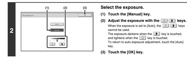
When using the document glass to scan multiple original pages, the exposure setting can be changed each time you change pages. When using the automatic document feeder, the exposure setting cannot be changed once scanning has begun. (However, when "Job Build" in the special modes is used, the exposure can be changed each time a new set of originals is inserted.)
