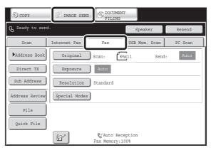
This screen only appears when the fax function and Internet fax function have been installed. The contents of the screen will vary depending on the devices that are installed.
