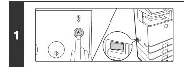
Press the [POWER] key ((()) on the operation panel to turn off the panel power, and then switch the main power switch to the off position.
