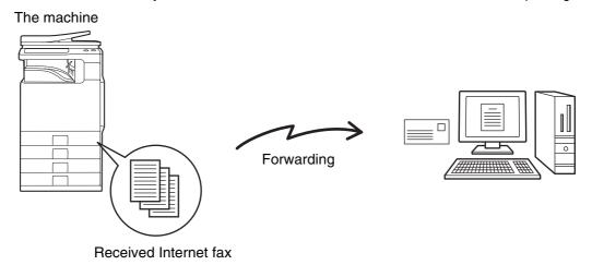
When faxes forwarded using this function are printed at the forwarding destination, the date and time of reception cannot be printed on the faxes. ("Receiving Date & Time Print" is disabled.)
