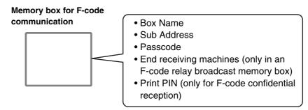
To use the following F-code communication functions, F-code memory boxes must be created in your machine: F-code confidential reception, F-code polling memory, F-code relay broadcast transmission
