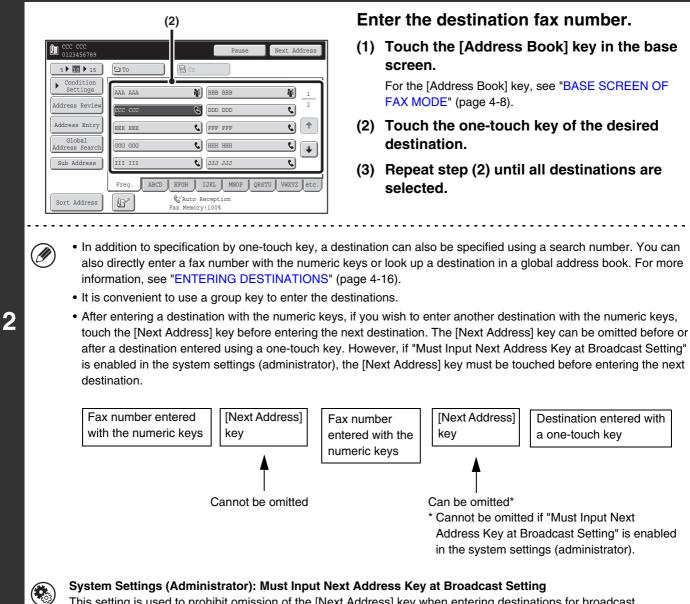
This setting is used to prohibit omission of the [Next Address] key when entering destinations for broadcast transmissions.
