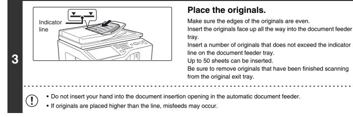
• Before inserting originals into the document feeder tray, be sure to remove any staples or paper clips.
