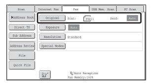
In the above screen, the scan size (the original size) is 8-1/2" x 11" (A4) and the send size is auto. If, for example, the scan size were 8-1/2" x 11" (A4) and the send size were 5-1/2" x 8-1/2" (B5), the image would be reduced before transmission.
