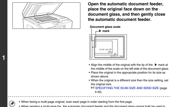
• When sending a multi-page fax, the automatic document feeder and the document glass cannot both be used to scan the original pages.
