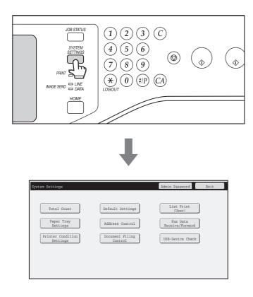
Make sure that the machine is in the standby state and then press the [SYSTEM SETTINGS] key on the operation panel.
