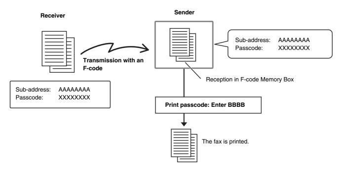
The F-code (sub-address and passcode) of the memory box to be used should be verified by the sender and the recipient before the fax is sent.
