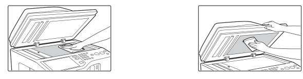
When wiping dirt off the machine, do not press down hard on the machine. This may damage or deform the machine.
