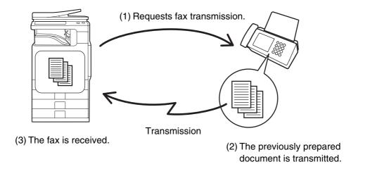
Make sure that an original is not placed in the machine when using the polling reception function.
