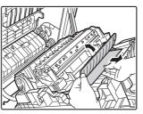
Open the right side cover, open the paper conveyor cover, and remove the paper.
