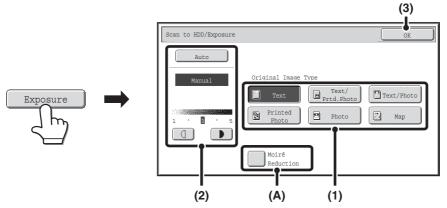
(1) Select the appropriate original type for the original to be scanned.
