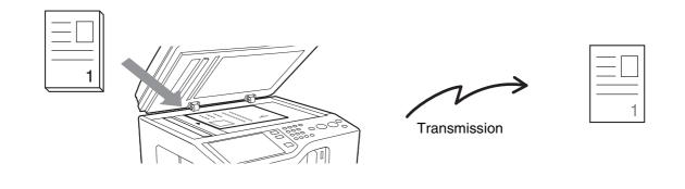
) When the document glass is being used for a transmission, Quick Online transmission will not operate.
