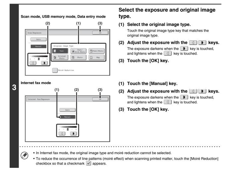
When using the document glass to scan multiple original pages, the exposure setting can be changed each time you change pages. When using the automatic document feeder, the exposure setting cannot be changed once scanning has begun.
