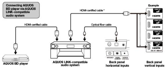
(EQ/LE650U/C6500U/LE642U series) Use HDMI IN 1 to connect ARC-compatible equipment.
