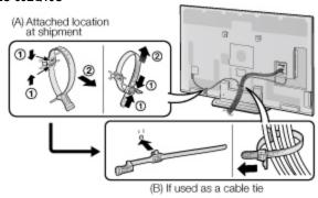
• The location of the AC cord holder differs depending on whether it is in its shipment location (A)or has been used as a cable tie (B).
