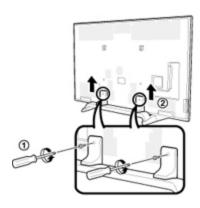
2 Unfasten the four screws used to secure the stand in place.
