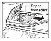
Open the document feeder cover and remove the paper feed roller.
