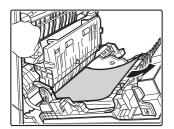
When opening the paper reversing section, open slowly and gently. Jerking the section open may cause the secondary transfer roller unit to detach, resulting in failure.
