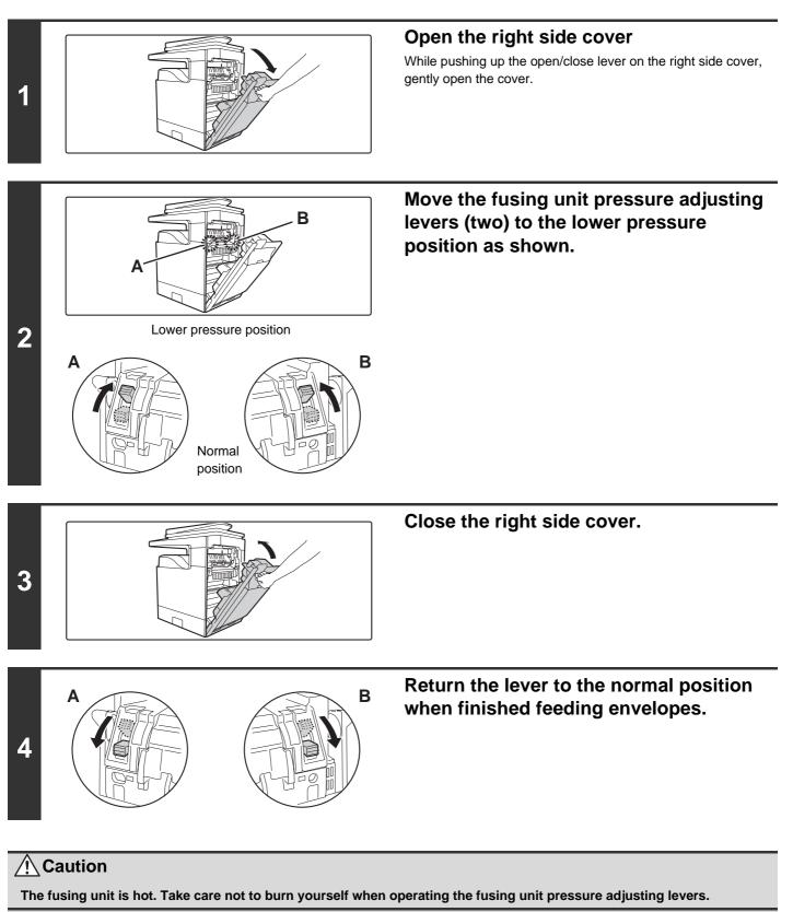
Be sure to return the levers to the "normal pressure position" before printing or copying on paper other than envelopes. Otherwise, fusing problems, paper misfeeds, or equipment failure may occur.
