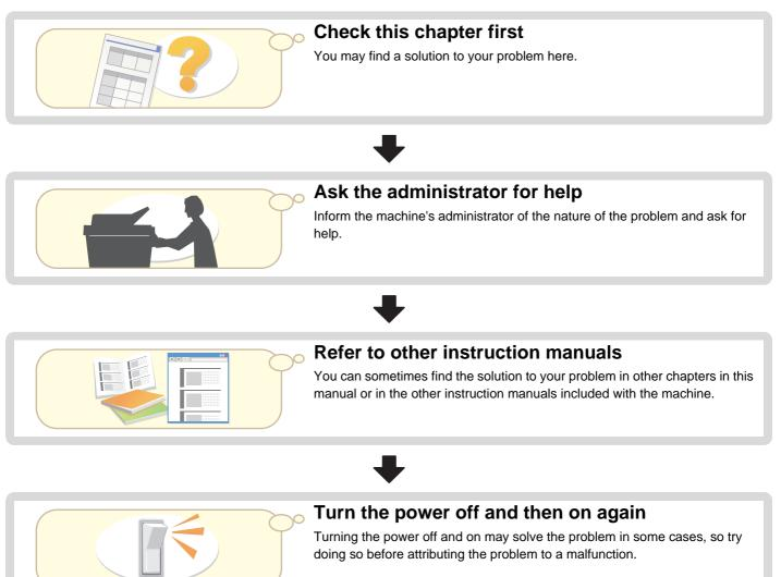
Press the [POWER] key ((0)) to turn off the power and switch the main power switch to the "off" position. Wait at least 10 seconds and then switch the main power switch and the [POWER] key (0) back on in that order.
