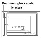
All originals should be placed in the left center position. Align the middle of the original with the tip of the **b** mark.
