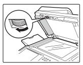
Open the automatic document feeder and remove misfeed originals while rotating the transfer roller in the direction of the arrow.
