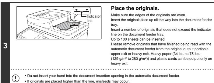
Before inserting originals into the document feeder tray, be sure to remove any staples or paper clips.
