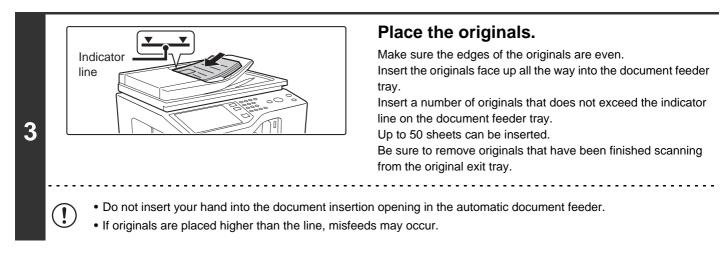
• Before inserting originals into the document feeder tray, be sure to remove any staples or paper clips.
