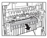
If a paper misfeed has occurred inside the fusing unit, press down on the green part, open the fusing unit, and remove the paper.
