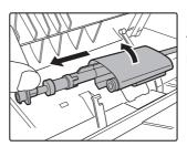
Remove the shaft rotating the roller cover upward and remove the shaft.
