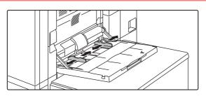
Adjust the bypass tray guides to the size of paper to be loaded.
