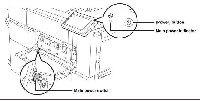
・When turning off the main power switch, press the [Power] button on the operation panel and then turn the main power switch to the " ()" position.
