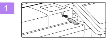
Connect the USB memory device to the machine.
