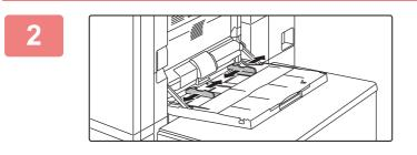
Adjust the bypass tray guides to the size of paper to be loaded.
