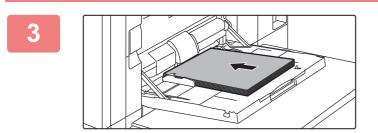
Insert the paper along the bypass tray guides all the way into the bypass tray until it stops.
