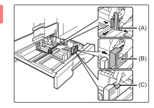
Adjust guide plates A and B by squeezing their lock levers and sliding them to match the longitudinal and transversal dimensions of the paper to be loaded.
